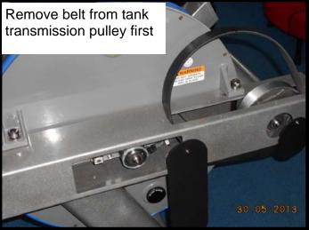
Once the tank is furthest forward, remove the belt first from the transmission pulley on the tank using care not to damage/move the sensor bracket/wiring.
