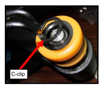
First, using a pair of C-clip pliers, removed the C-clip holding the seat wheel onto the axle. Behind the C-clip is another washer. Then, remove the wheel itself (this can sometimes take a little persuasion). Behind the seat wheel there are 3 washers (spacers) that make up the gap between the rear of the seat wheel and the seat frame bearing.
