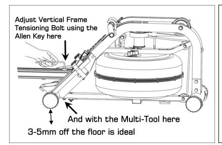
Close up view of the Vertical Seat Rail Tensioning Bolt M10 Nyloc location.
