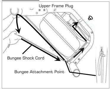
Move the Rowing Handle to it's farthest forward point on the Mainframe, then cut the plastic end tie and follow the drawing above for bungee removal.
