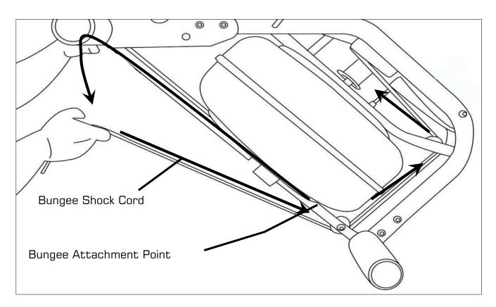
1.To detach belt, simply pull beyond the range of the normal rowing stroke until the belt detaches from the Belt Bungee Pulley.
