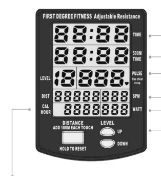
**CAL HOUR:** Calories burned per hour at the current Watts. Shows total calories burned when exercise is stopped.
