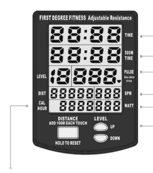
**CAL HOUR:** Calories burned per hour at the current Watts. Shows total calories burned when exercise is stopped.
