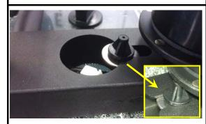
Install the Speed Sensor as shown.
