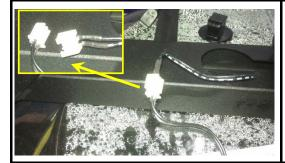
Disconnect the sensor cables
