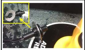
Remove the washer from the Speed Sensor
