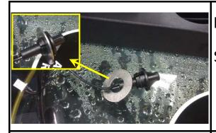
Fit washer onto the new Sensor
