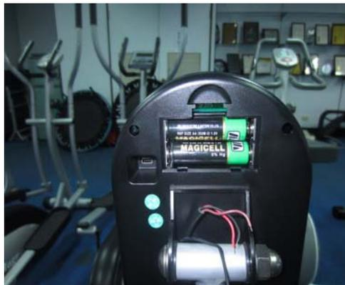
STEP 2: Check Sensor Connector at rear of Monitor
