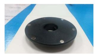
3. Check sensor head – the internal sensor should be no more than a few millimeters inside the hole
