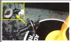
Remove the washer from the Speed Sensor
