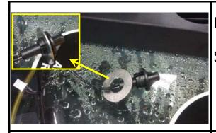
Fit washer onto the new Sensor
