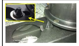
Pull the Speed Sensor out of the frame
