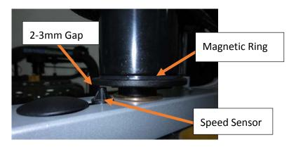
2. Visually check all 6 magnets in the magnetic ring are present and flush (no need to remove the ring)
