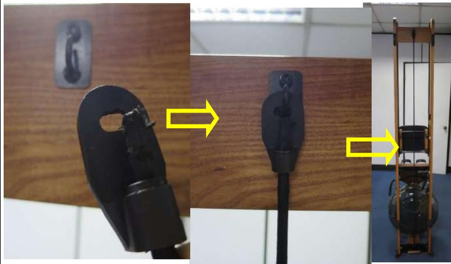
Hook it on the bracket on the rear board.
