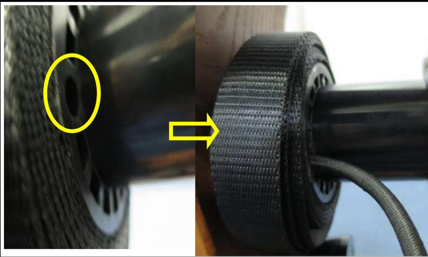
Thread the new bungee into the pulley
