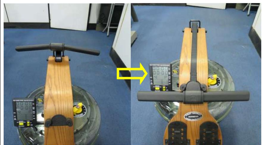
Replace the handle onto the bar catches.
