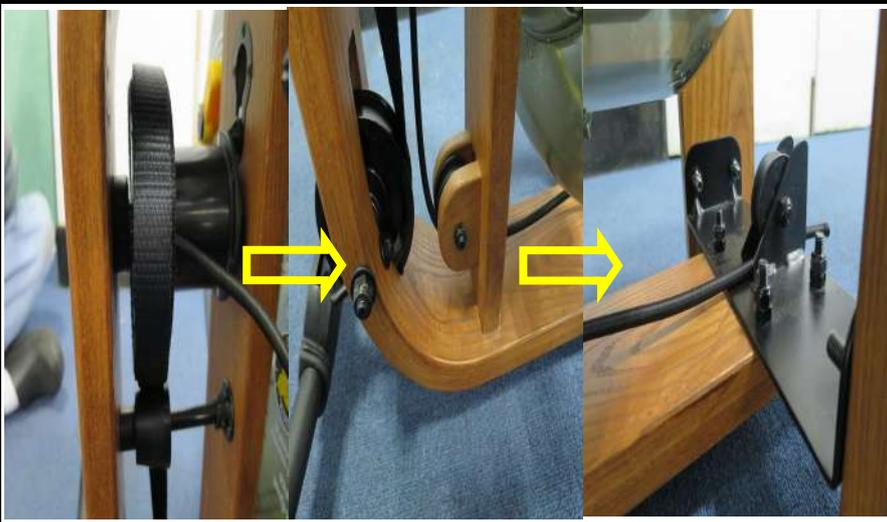
Rotate the Belt and make sure it is secured. The thread the bungee over the top bungee pulley to the lower bungee pulley
