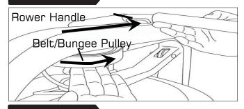
Wind the Rower Belt onto the Belt/Bungee Pulley until the Rower Handle is as it's furthest forward position.
