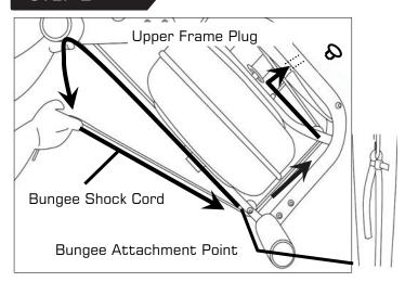
Move the Rowing Handle to it's farthest forward point on the Mainframe, then cut the plastic end tie and follow the drawing above for bungee removal. Next, remove the Upper Frame Plug to allow the Bungee Shock Cord to be threaded through the top of the frame. Note: You will need to rotate the Belt/Bungee Pulley to align the holes properly. Should the belt drop off of during the bungee change, please refer to the previous
