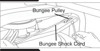
Rethread the Bungee Shock Cord (on opposite side of the Idle Wheel) back through the Bungee Pulleys and tie off at the Attachment Point.
