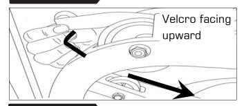
Begin reattaching the Rower Belt by threading around the Rower Belt Pulley with the Velcro side facing upward as illustrated.
