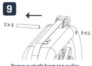
Remove shaft from top pulley
