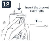
Using the longer bolt provided, bolt the bracket to the frame. Align Tablet Holder bracket and fully tighten all bolts.
