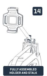
Test your device is held firmly in place now, and before any exercise session. If your device is being left in place between exercise sessions it is recommended that the device is lowered to rest on the frame of the rower until you reposition and test before
