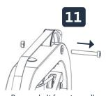
Remove bolt from top pulley
