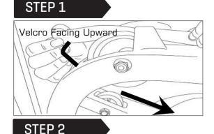
Begin reattaching the Rower Belt by threading around the Rower Belt Pulley with the Velcro side facing upward as illustrated.
