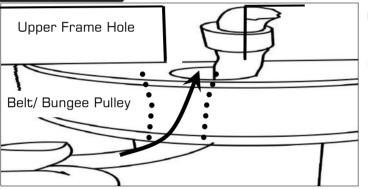
Once Bungee Cord and Upper Frame Hole are aligned, push the Bungee Cord up and through the frame as shown
