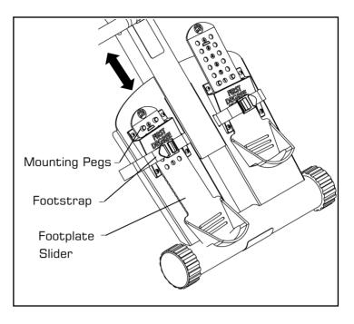
WARNING: Never operate this Rower without feet properly secured in Footstraps, or without the sliding portion of the Footplate Slider locked into position!
